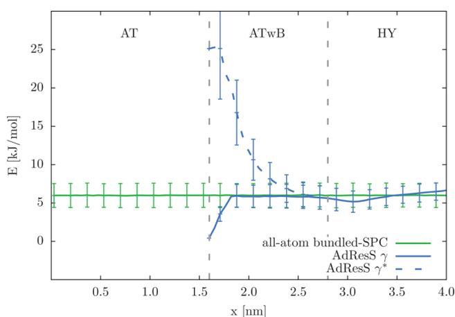
**Figure 8.** Average bundling energy of a bundle ( $U_B$ ; eq 3) with standard deviations along the direction of the resolution change. The results are plotted for the AdResS simulation and reference all-atom simulation of bundled-SPC water (with changed Lennard-Jones parameters according to ref 32). The AdResS profile is computed separately for the  $\gamma$  and  $\gamma^*$  functions (eqs 4 and 5, respectively). Resolution region boundaries are denoted with the vertical gray lines.
