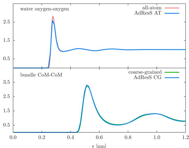
**Figure 6.** Radial distribution function (RDF) of oxygen atom (top) and bundle CoM or CG beads (bottom). The AdResS simulation results (AdResS AT and AdResS CG denote the region where the calculation is performed) are compared to the RDFs from reference all-atom and coarse-grained simulations to point out that the local structure is well reproduced.
