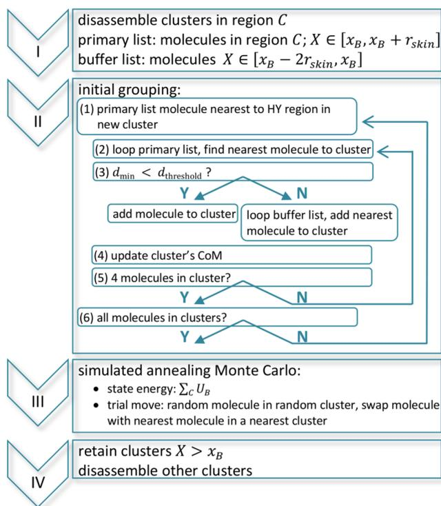
Figure 2. Flowchart of the SWINGER algorithm.
